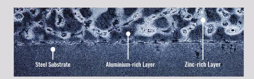
ALZU® steel uses its alloy coating of Aluminium and Zinc to achieve excellent corrosion resistance performance and surface appearance. The ALZU® steel coating forms an interlaced mesh structure of Aluminium and Zinc. The Zinc-rich areas are the first line of defence in protecting the steel substrate, while the Aluminium-rich layer provides the second line of defence. These two layers work together to provide superior corrosion resistance performance for roofing and walling products.
