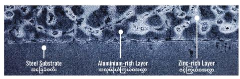
ALZU® steel uses its alloy coating of Aluminium and Zinc to achieve excellent corrosion resistance performance and surface appearance. The ALZU® steel coating forms an interlaced mesh structure of Aluminium and Zinc. The Zinc-rich areas are the first line of defence in protecting the steel substrate, while the Aluminium-rich layer provides the second line of defence. These two layers work together to provide superior corrosion resistance performance for roofing and walling products.
