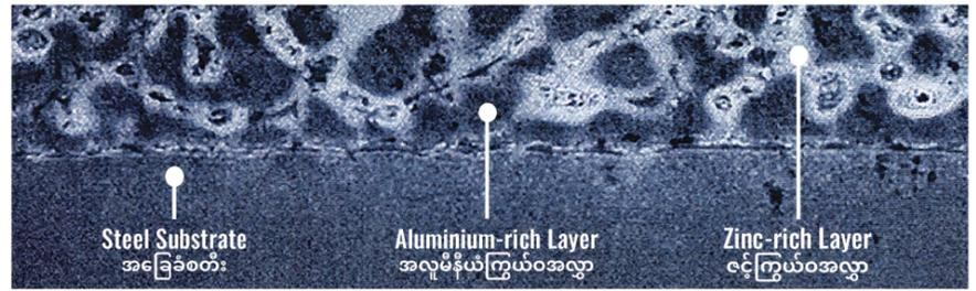
ALZU® steel uses its alloy coating of Aluminium and Zinc to achieve excellent corrosion resistance performance and surface appearance. The ALZU® steel coating forms an interlaced mesh structure of Aluminium and Zinc. The Zinc-rich areas are the first line of defence in protecting the steel substrate, while the Aluminium-rich layer provides the second line of defence. These two layers work together to provide superior corrosion resistance performance for roofing and walling products.
